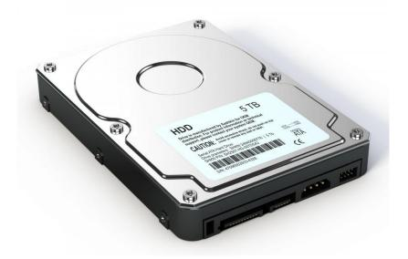
This is your computer's hard drive, and it is on this device that all your information is stored. There will be two cables at the back of this device. Unplug them, then unscrew the mounting screws and remove the device.
